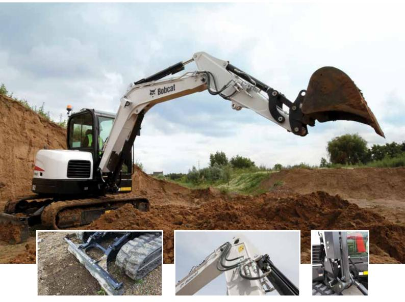
The floating blade feature is standard for the product range, allowing each operator a perfect levelling result.
